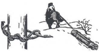
*Timber Hitch* - Used in hauling timber and for commencing the diagonal lashing.
